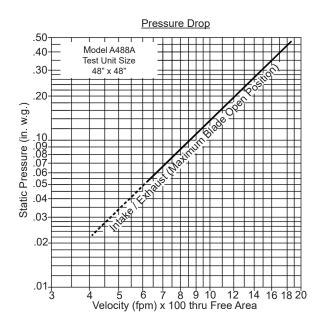
The AMCA Certified Ratings Seal applies to Air Performance only. Tested in accordance with AMCA 500-L Test Figure 5.5-6.5
